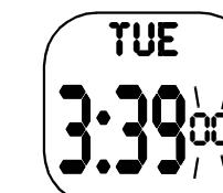
When setting the seconds, press ADV./ST./SPL. to reset them to 00. Press or hold down ADV./ST./SPL. to advance through the digits or toggle between 12- or 24-hour display, then press SET/LIGHT/STP/RST. to confirm.
